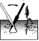
Push handle of bar forward to firm soil at top of roots
